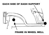
Install the three (3) routing clips (G) along the length of the supply tubes at the locations shown above. See further instructions below.
